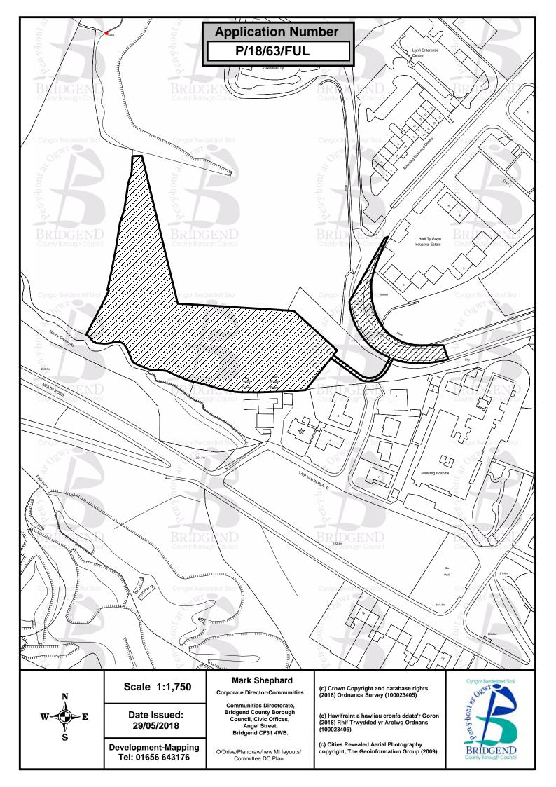
The proposed building is to be positioned at the far eastern corner of the field and is to be accessed via an extended access track (approximately 150m in length) that runs along the northern boundary of the site and connects the barn and the access off the industrial estate access road. The access road is to be finished in a loose bound permeable material to match the hard standing area.
